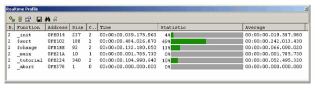
Figure 5.130 Realtime Profile window (function profile)
